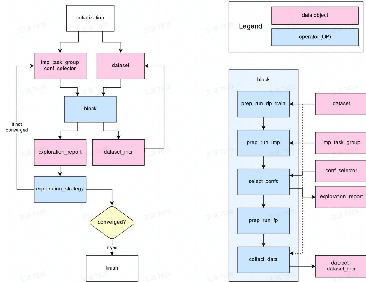
In the center is the **block** operator, which is a super-OP (an OP composed by several OPs) for one DP-GEN iteration, i.e. the super-OP of the training, exploration, selection, and labeling steps. The inputs of the **block** OP are **Imp\_task\_group**, **conf\_selector** and **dataset**.
